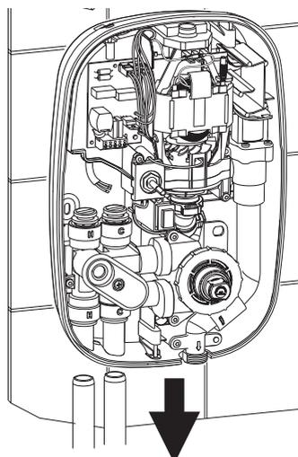
**Important!** This Mira Event XS **must** be fixed to the wall at all three fixing positions. The fixing holes are elongated to assist in vertical and horizontal alignment.
