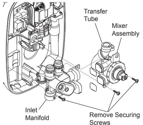
**5.9.** Inspect inlet manifold/valve interface seals and renew if required.
